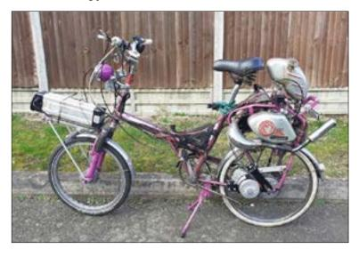
was a bit of a problem, but as a temporary fix I mounted it on the front carrier. I decided to use a thumb switch accelerator control as the bike has a twistgrip accelerator and I envisaged that I would twist the throttle open and then push down with my thumb to get electric LPA, hopefully!
