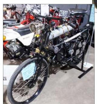
Derek Langdon's 1923 Atlas (left) is a wonderful construction, made to the highest engineering quality as is always the case with Derek's machines. The 142.5cc two-stroke engine has a chain-driven magneto and was made by Aston Motor & Engine Co.
