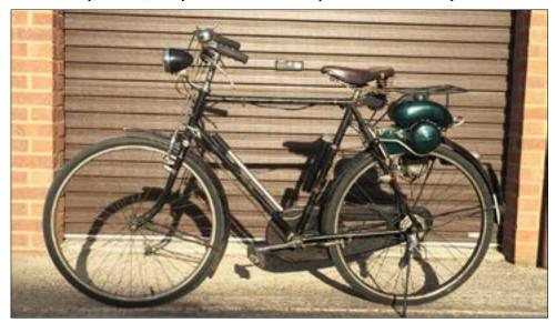
...to set up and that you're better off without it.\* Drive is transmitted from the two-stroke engine to the rear wheel by means of a carborundum-faced roller. Three engagement positions are possible: disengaged, engaged and a third position to compensate for underinflated or worn tyres. This is also useful in wet weather when roller slip can be a problem. Riding a non-Synchro Power Pak requires a degree of anticipation - I have to remember to be in first
