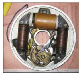
When I previously replaced the coil I had tested the capacitor in-situ but I had not got a replacement at that time. So now in lockdown with plenty of time on my hands I decide a complete rebuild of the magneto was needed. The pictures show the strip down all the way to the capacitor, which is buried in the back of the contact breaker housing, affixed by studs through the backplate of the magneto.
