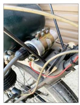
(\*The main problem with a Synchromatic clutch is lack of enough travel in the factory-supplied twistgrip throttle-cum-clutch control. The clutch doesn't fully release even with the cable correctly adjusted, so it drags at idle when stationary, usually stalling the engine. Fitting a clutch lever cures this completely - as it has on my Synchromatic, now a pleasure to ride! Ed.)
