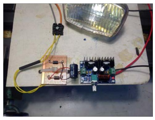
The LEDs I've been experimenting with are really for tail-lights so they won't focus, but more suitable ones are probably available. In any case the exercise was to make the bike more visible in daylight. The photo shows the test rig in the lathe, next comes the rectifier, then the smoothing capacitor (which didn't work) and the little Chinese DC/DC regulator. I must warn you that this set-up has not been road tested, and remember nothing breaks on the drawing board!
