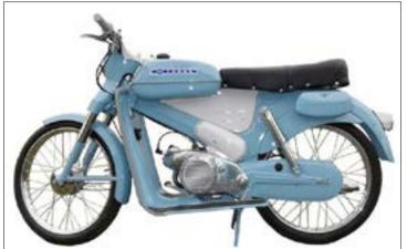
Left, a full-house, Puch-engined Tomos Colibri T12, with foot-plates, leg-guards dualseat, valanced rear mudguard, tool boxes and an in-fill panel in the frame.
