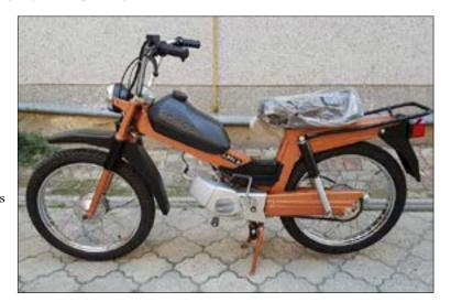
In the early 1990s Tomos launched a new engine, the A35 unit, which replaced the earlier A3 (seen below), though they are effectively the same and had but a few minor changes. It was a 49cc 38mm x 43mm unit with reed-valve induction, a high 9.1:1 compression ratio and two-speed automatic gearbox, and was fitted to the Sprint, Targa and Targa LX.
