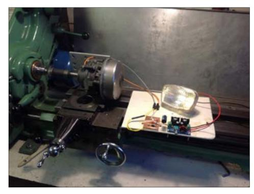
The output of the mag is, of course, AC with voltage and frequency varying with electrical load and engine speed. This is not what an LED would like, so putting the output through a rectifier was the first move to turn it into DC which the LED does like.
