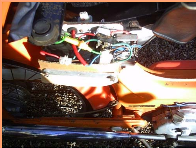
Dave Watson went all the way to Swindon to buy this Honda PC50 that has been converted to Battery Coil Ignition
