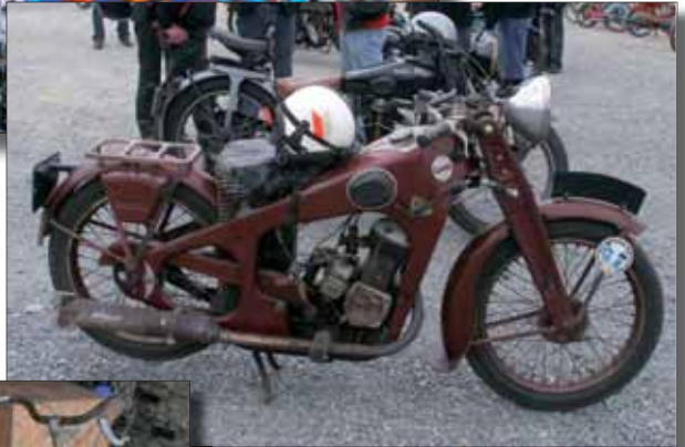
Left- 1952 Alcyon 50cc cyclomoteur with ABG Vap engine, made in Courbevoie, very typical of the multifarious marques which flourished in the late 40's to early 50's, only to be swept away by the runaway success of Motobécane's Mobylette.
