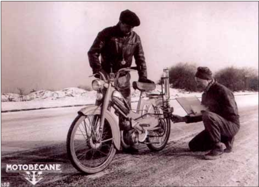
(Motobécane's engineers checking fuel consumption of an AV85 at Montlhéry during the hard winter of 1961-62. photo courtesy MBK & Patrick Barrabès)
